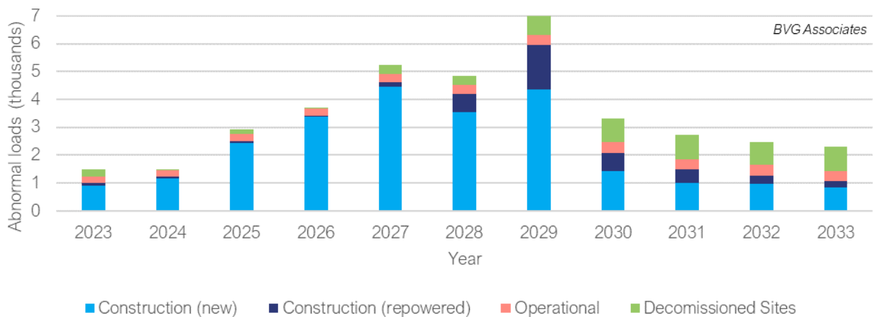
Figure 7: Abnormal load movements required to 2033, Enhanced Pipeline Scenario plus 50% Repowering.
