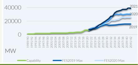
Plans will see an increase in current B6 boundary capacity almost threefold, to 15GW by 2030, in half the time it took us to increase boundary capability [threefold] to 6GW
