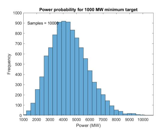
Figure 4 Distribution of additional installed capacity based on setting a Seismic Impact Limit of 0.00809 nm/MW<sup>-0.5</sup> based on 10,000 randomised simulations. The position, size and capacity of each wind farm was assigned randomly in each iteration of the simulation.
