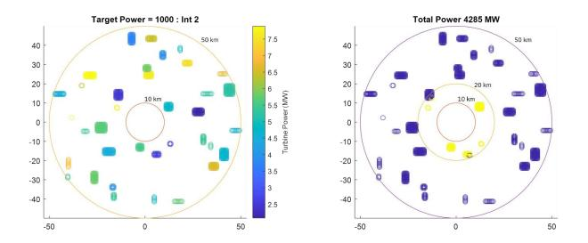
Figure 3 Example of a single iteration. Left: showing the random placement of wind farms that have been assigned turbines with randomised power output (between 2 and 8 MW, see colour bar). Right: Farms coloured blue are below the Seismic Impact Limit, while farms in yellow have their seismic output capped at the Seismic Impact Limit (likely via some form of seismic mitigation).
