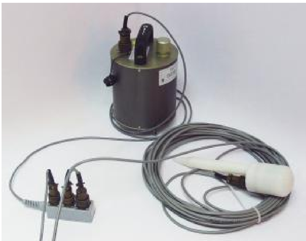
Figure 15 - Guralp 6TD, GPS and cabling.
