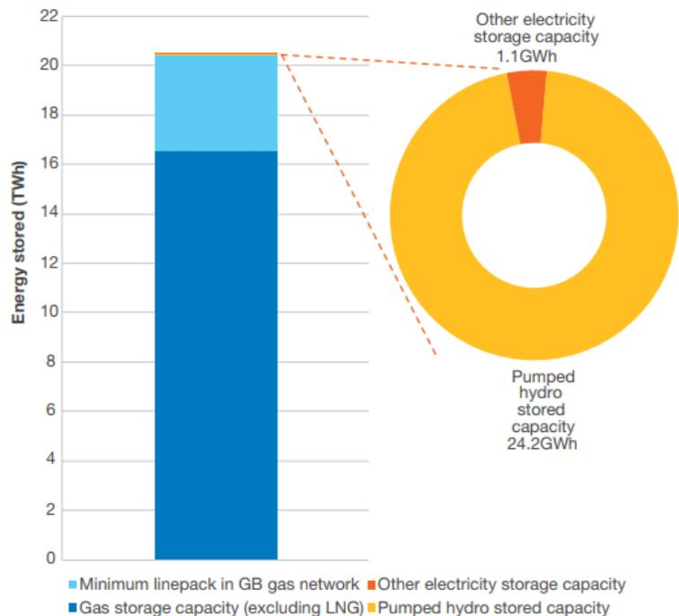
At the end of 2020 there was approximately 15,000 GWh of gas in storage, and a minimum 3,800 GWh of linepack in the gas network; there is less than 30 GWh of electricity storage capacity, of which 96% is from pumped hydro storage sites, with around 4% from other forms like batteries.
