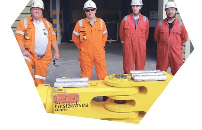
The connector allows the mooring lines to be prelaid on the seabed prior to the arrival of the wind turbine structure, eliminating the need for expensive construction vessels and significantly reducing installation times. The technology is now being used at hundreds of facilities around the globe.
