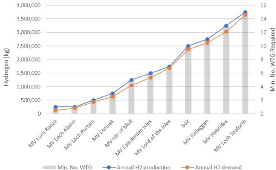
Wood's energy modelling, in collaboration with CMAL and Siemens-Gamesa, has determined the size of wind farm required to produce enough hydrogen for each ship operating the ferry routes (SWT-DD-130 4.3 MW).
