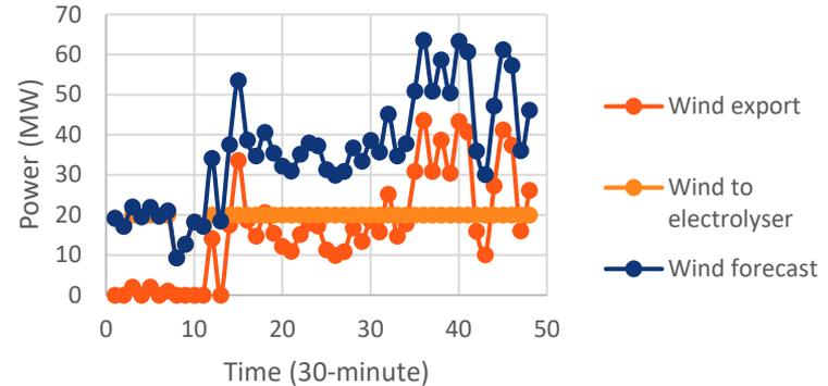
When wind power is above 20MW, i.e. above the maximum electrolyser capacity, power to the electrolyser is prioritised and the remaining wind power is exported to the grid.
