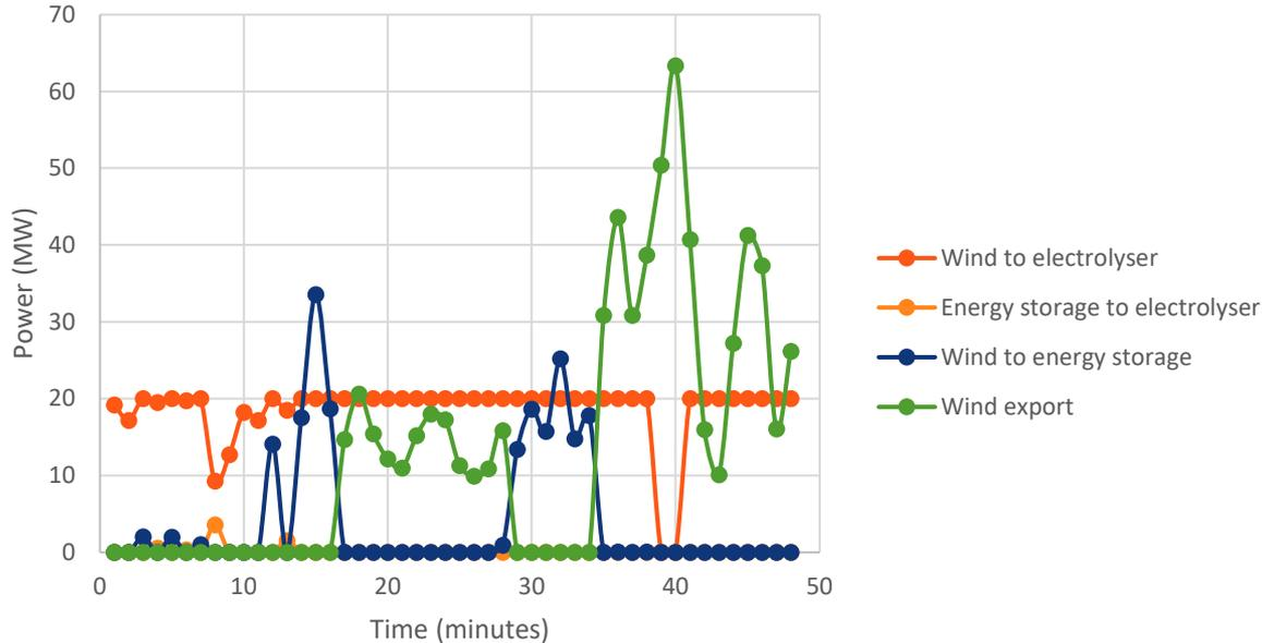
When wind power is above 20MW, power to electrolyser is prioritised and the remaining goes to the energy storage unit, as e.g. at HHs 28-35. The store is then full and discharges at HHs 39-40 when higher prices occur
