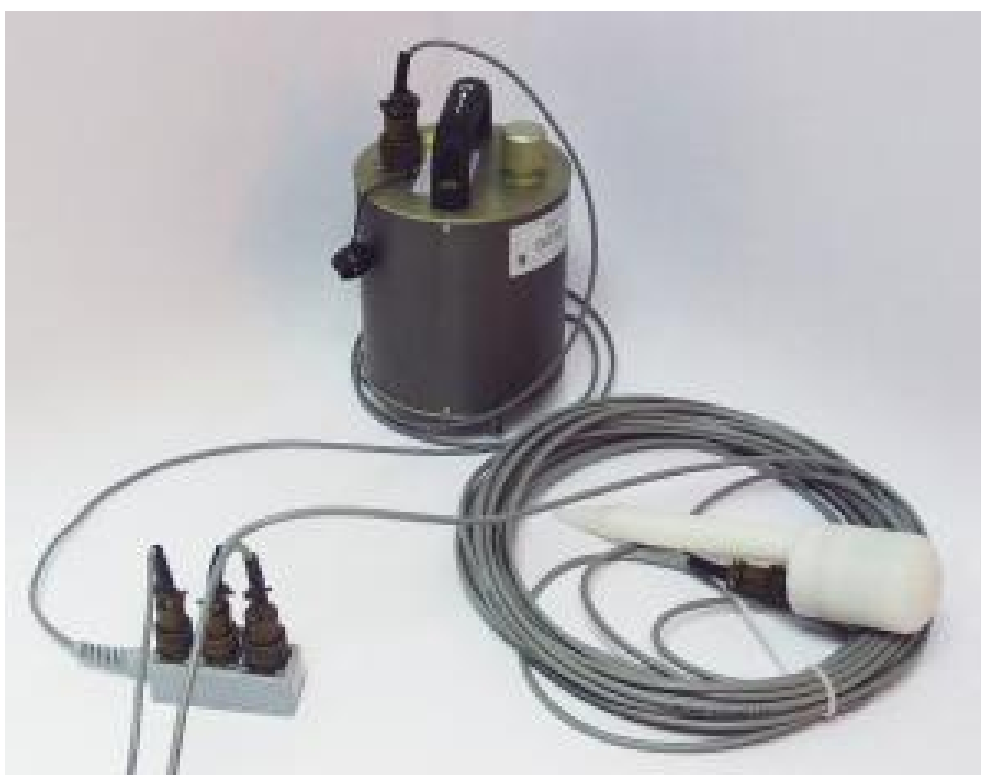
Figure 15 - Guralp 6TD, GPS and cabling.
