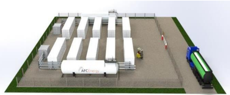
Multi-MW Rendered Off Grid Fuel Cell Installation
