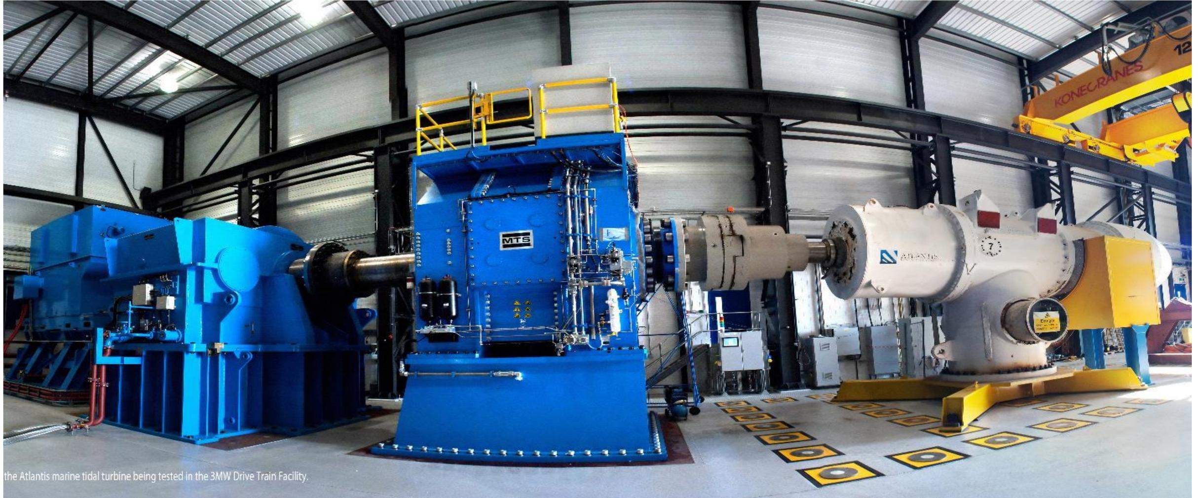
the Atlantis marine tidal turbine being tested in the 3MW Drive Train Facility.
