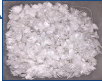
“Regenerated” fibres Fluidised bed recycled glass fibres
