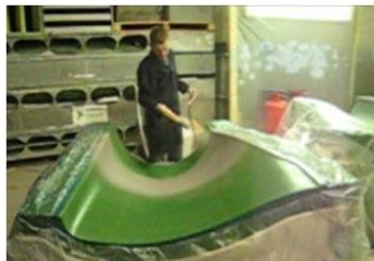
Surface coat being applied.
