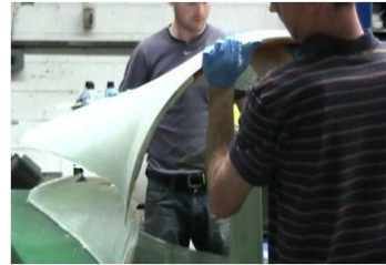
Top skin pre-form being placed on top of shear web
