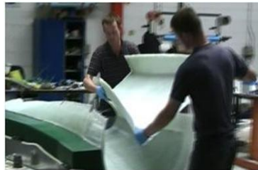
Shear web pre-form being placed in position
