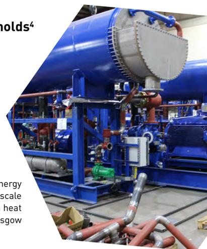
Star Renewable Energy manufacture large scale heat pumps for use with heat networks in Glasgow
