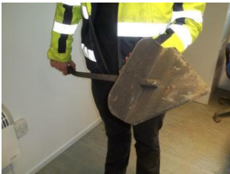
A peat cutting spade is an effective way for non-invasive silt fence erection avoiding unnecessary digging.
