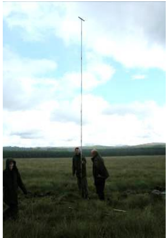
Peat probing very deep peat. Thorough site investigation, such as detailed peat depth surveys, is essential at the early stages.
